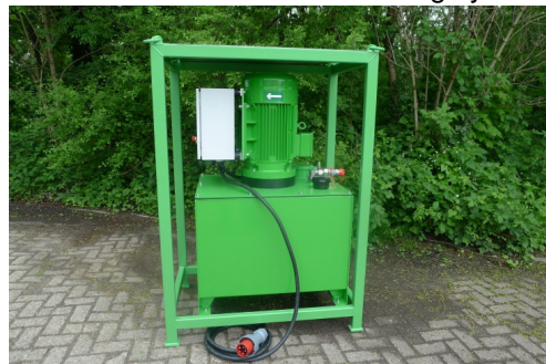
Electric-hydraulic power-pack with offshore specifications
