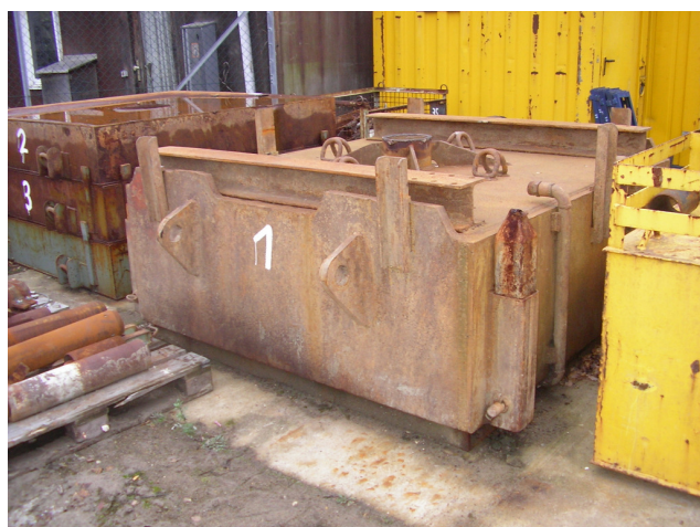
Ballast block for standpipe
