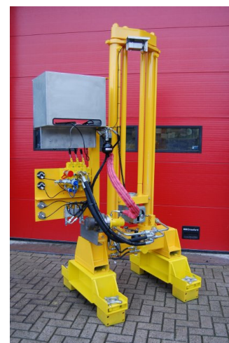
Hydraulic gripping system for quick lowering and retrieving of the tubes
