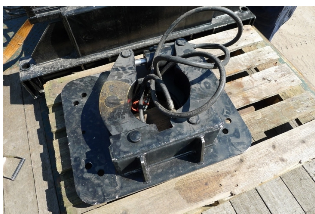
Hydraulic clamp to hold the standpipes in place
