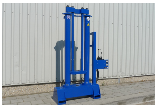
350 kN CPT penetrometer pusher
